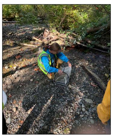
ZoAnn from Streamkeepers explained the procedure to John and Quirien, then introduced the D-net and described how to set it the creek bed. The net mouth is 30 cm wide and the sample area was a 30 cm square, measured by ruler. Quirien held the net in place while John examined the underside of a stone he had removed to make way for the net. The underside of this pebble had a number of Caddisfly larvae attached.
